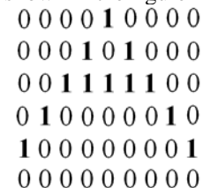
Figure 2: ASCII ‘A’ image in 9X6 cellular matrix
